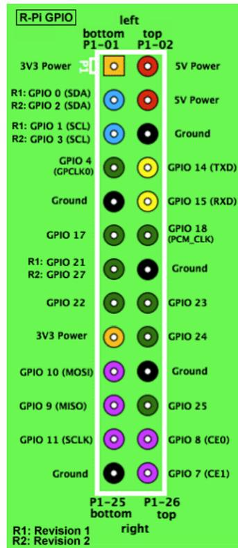
**Figure 10:** Broadcom GPIO pin assignments. (Image from [2])
